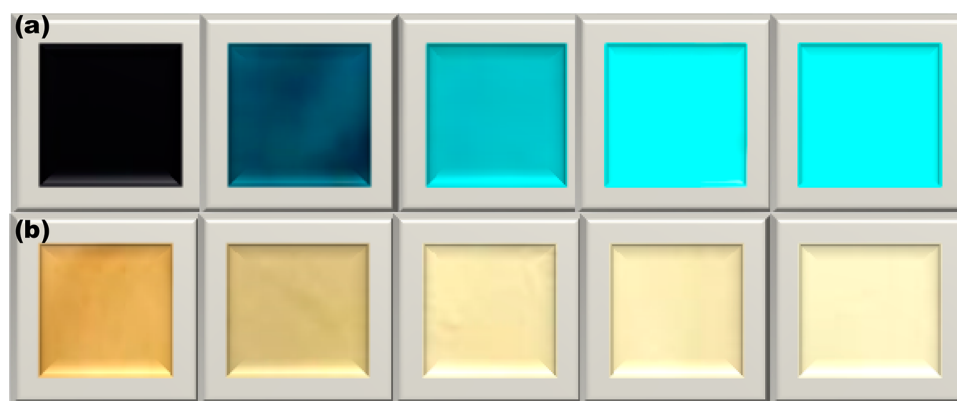
Figure 3. Visual colorimetric detection of TNT. Photograph of the fluorescence quenching of FNFMs treated with different concentrations of TNT in aqueous phase when viewed under UV ( \lambda_{\text{ext}}=254 nm) (a) and daylight (b). The tested TNT concentrations are 5 \times 10^{-3} , 5 \times 10^{-4} , 5 \times 10^{-5} , 5 \times 10^{-6} , and 5 \times 10^{-7} M from left to right. The color of the membrane changes from bright bluish-green to blue with increasing concentration.
